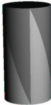
Figure 3.17: A cylinder represented as a NURPS surface. The different patches have been shaded in different shades of gray.
