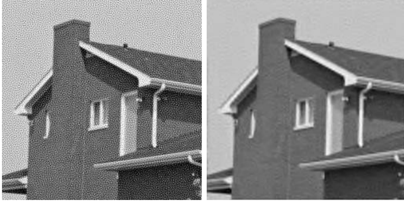
Figure 5.10: Left: an image with artificial, correlated noise. The noise is the result of a convolution of white noise with FIR highpass filter. Right: the result after level-dependent wavelet thresholding. We use biorthogonal filters with four primal and four dual vanishing moments and filter lengths 7 and 9. Signal-to-noise ratio rises from 4.97 dB to 16.83 dB.
