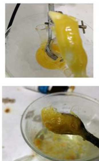
Figure 2. Gel formation as a result of the polymerization reaction of PPTA in [C_8MIM][Cl] at 0 °C.
