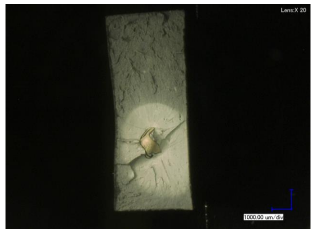
Figure 4. Fracture surface with impurity.
