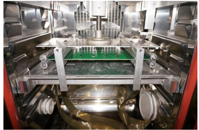
Figure 2: Realization of the four point bending setup in the thermal chamber
