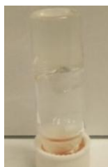
Figure 6.4 Rheopectic gel formation of 10 wt% [P_{444}E_3][DOSS] in water upon shaking at 0 °C.
