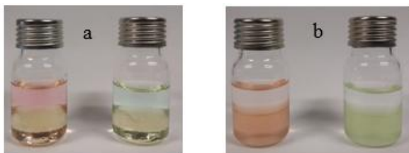
Figure 6.18 Picture of Sm/Co pair (pink on the left) and La/Ni pair (green on the right), before (a) and after (b) extraction.
