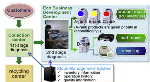
Fig. 2. Ricoh's reuse and recycling system.
