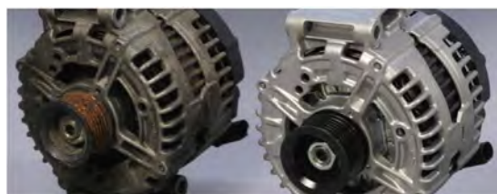
Fig. 4. Example of core and remanufactured product.
