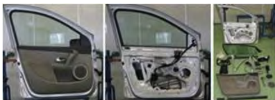
Fig. 6. Car door disassembly and remanufacturing.
