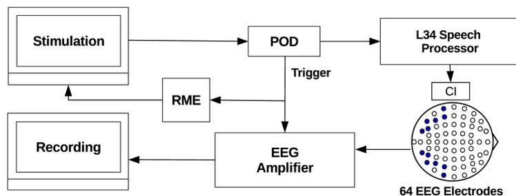
Figure 1: Schematic representation of the measurement set-up. The EEG amplifier is a Biosemi ActiveTwo EEG Recording System with a sample rate of 8192 Hz. The subject is seated in an electrically-shielded sound-proof booth.
