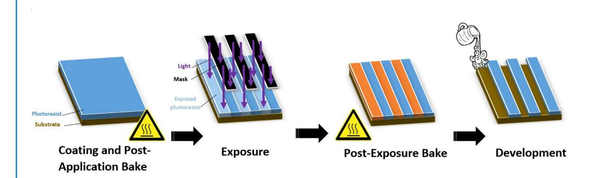
In the process of photolithography, a photoreactive polymer, called photoresist, is spin coated on a wafer, solvent is removed by a bake step, then the wafer is exposed to light through a patterned mask. This activates photo-acid generator (PAG) molecules, that then catalyse a cleavage reaction during a post exposure bake (PEB) step. This cleavage of functional groups leads to a change of the hydrophilicity of the polymer, and thus of their solubility in solvent.
