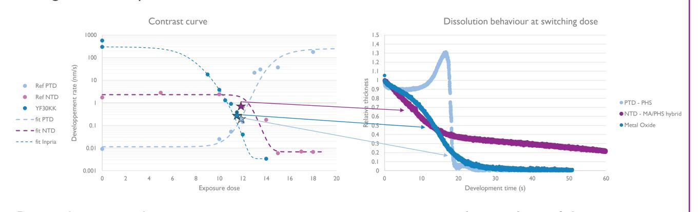
But we have seen that just comparing contrast curves is an uncomplete analysis of the dissolution properties of a resist, because different resist platforms show very different dissolution curves at switching dose. We believe that a better understanding of these different behaviours should help the resist design and lead to resists with better performances.
