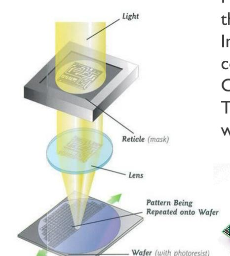
For all advanced microelectronic chips produced nowadays, the patterning of the electronic circuit on silicon is realized through various steps of photolithography, a process during which light is used to print a pattern on a substrate. In the past decades, the miniaturization trend predicted by Moore's law has required photolithography to use light with continuously shorter wavelength in order to print smaller critical dimensions.
