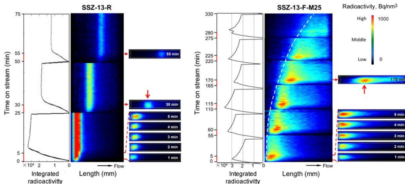
**Figure 6.** Positron emission tomography image series of (left) SSZ-13-R and (right) SSZ-13-F-M25 for  $^{11}\text{C}$ -CH<sub>3</sub>OH MTO reaction. Three  $^{11}\text{C}$  methanol pulses were delivered to SSZ-13-R and six to SSZ-13-F-M25 (marked with red dashes). The radioactivity is decay-corrected in each slice along the catalyst bed ( $T = 350\text{ }^{\circ}\text{C}$ ;  $\text{WHSV} = 0.5\text{ g g}^{-1}\text{ h}^{-1}$ ).
