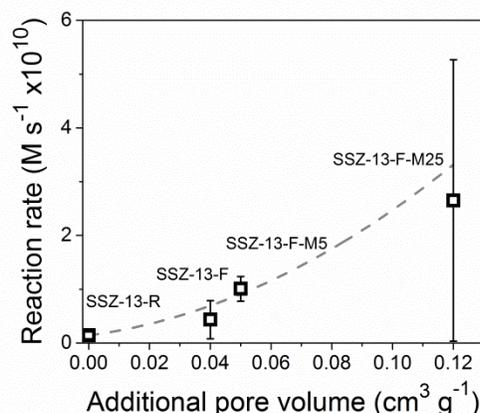
**Figure 5.** Averaged reaction rates ( $\text{mol L}^{-1} \text{s}^{-1}$ ) independently observed for at least 4 different SSZ-13 crystals over 3000 frames (corrected to remove reappearing individual catalytic events) detected by NASCA analysis vs. the extraframework, non-CHA, pore volume derived from Ar physisorption.
