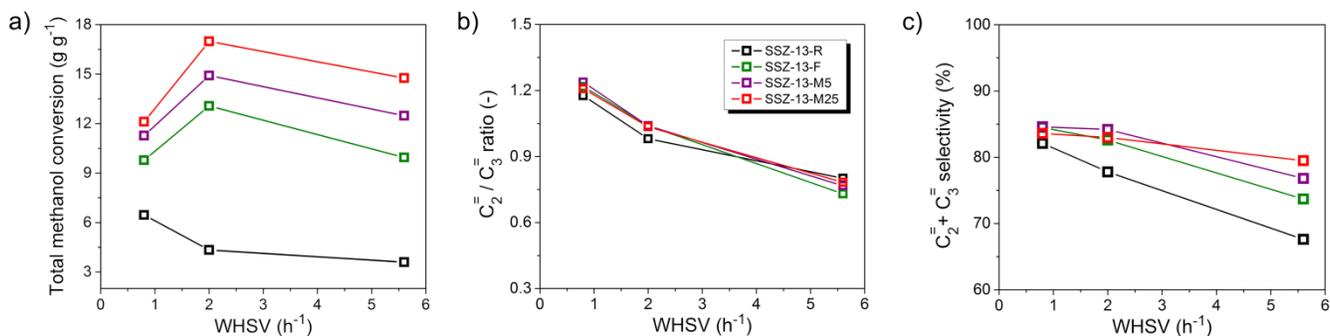
**Figure 2.** Influence of WHSV on the catalytic performance of the studied SSZ-13 catalysts: (a) total amount of methanol converted after 24 h time on stream, (b) ethylene/propylene ratio and (c) total ethylene + propylene selectivity at a methanol conversion of 98%.
