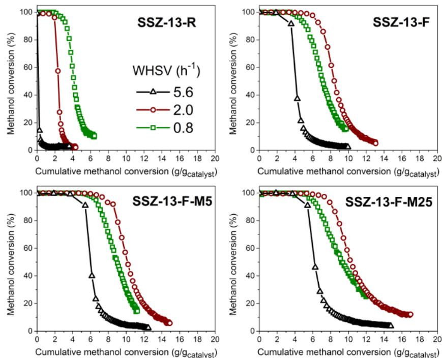
**Figure 1.** Methanol conversion as a function of the cumulative amount of converted methanol for different WHSV. Conditions: 350°C, 50 mg of catalyst, atmosphere pressure, 24 h.
