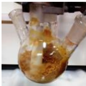
Figure 3. Reaction mixture after a polymerization reaction in a [2-Me-C 6 Pyr][Cl]/NMP solvent mixture. The chloride anion successfully prevented precipitation of the growing polymer chain in the early stage of the reaction and a gel in the form of a solid crumble was formed.
