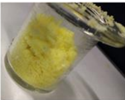
Figure 1. Reaction mixture after polymerization reaction in the presence of a base performed in a cylindrical reaction vessel. The polymer and reaction mixture have formed a solid, yellow crumble.
