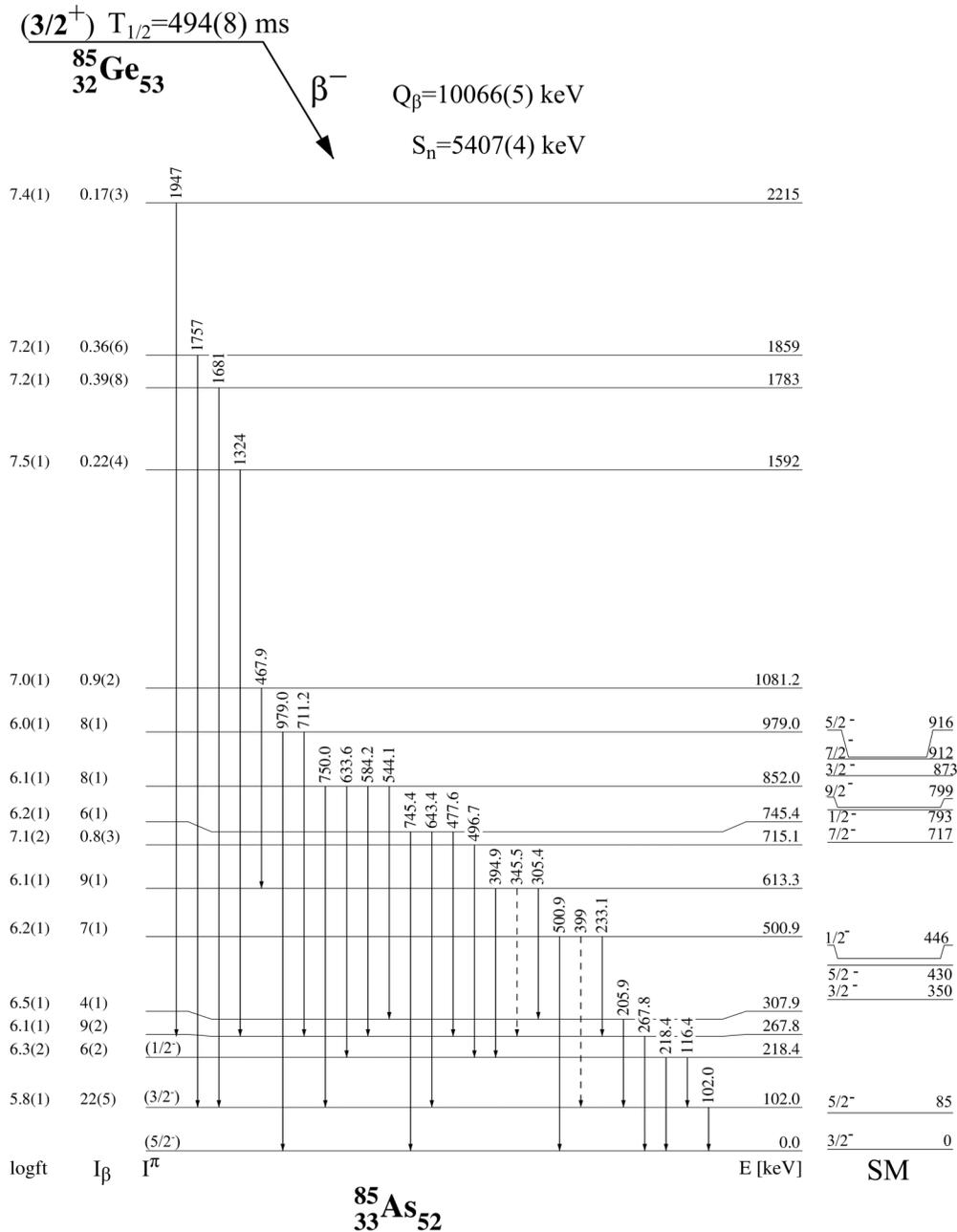
FIG. 3. Partial decay scheme of  $^{85}\text{Ge}$  as obtained in this work. Dashed transitions were tentatively assigned on the basis of weak  $\beta$ - $\gamma$  coincidence. The  $Q_\beta$  and neutron-separation  $S_n$  energy were adopted from Refs. [20,21], the half-life is taken from Ref. [8]. Listed  $\beta$ -feeding intensities were obtained as “apparent,” i.e., assuming no direct feeding to the  $^{85}\text{As}^{\text{g.s.}}$ ; compare text.
