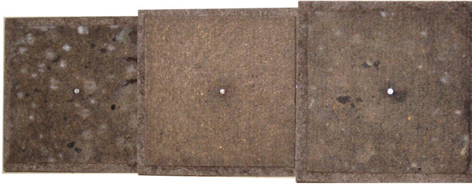
Figure 13. Mold growth on weight specimens of FIBREBOARD 2 at the end of step 4 (left to right: top, middle and bottom specimen)
