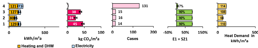
Figure 7. The data analysis of building stock by cluster shows the far better similarity of the buildings than an analysis by construction year.
