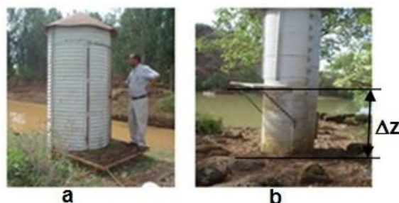
Figure 6. Automatic water level recorders installed by USBR in 1959, and photographed in June 2012 along the alluvial Gumara River (a; at 11.838408°N, 37.637086°E) and the bedrock Abay River 4 km downstream from Chara-Chara weir at the outlet from Lake Tana (b; at 11.567543°N, 37.403952°E). \Delta z indicates the depth of sediment that was accumulated in Gumara's natural levee over the intermittent 53 years, i.e. 140 cm (after Abate et al. (2015)).
