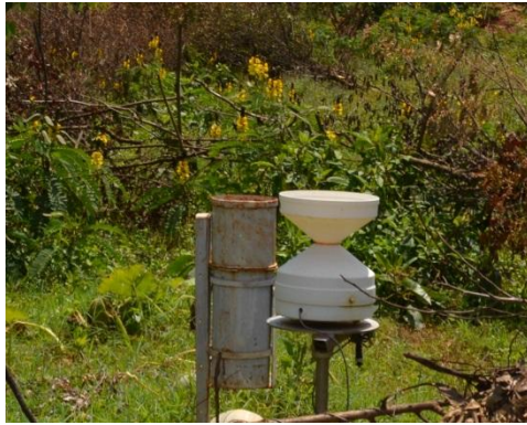
Figure 2. Typical manually recording rain gauge and e+ RAIN logger installation in Wanzaye area
