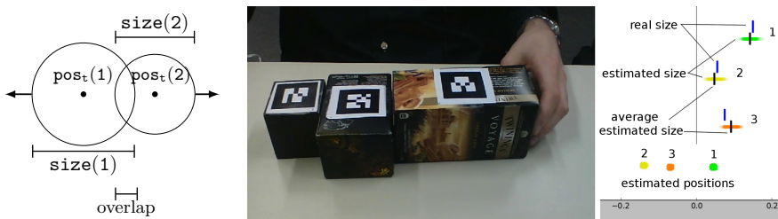
Figure 4.11: Learnsize scenario. Sketch on the left: the objects are pushed away from each other when they overlap, applying a displacement. Picture on the center with 3 objects. The right figure represents the estimated objects' positions (yellow, orange and grey), and the estimated size (one point per sample) using artificial dynamics. The blue lines are the real size and the black lines the average estimated size. The distance is measured in meters.
