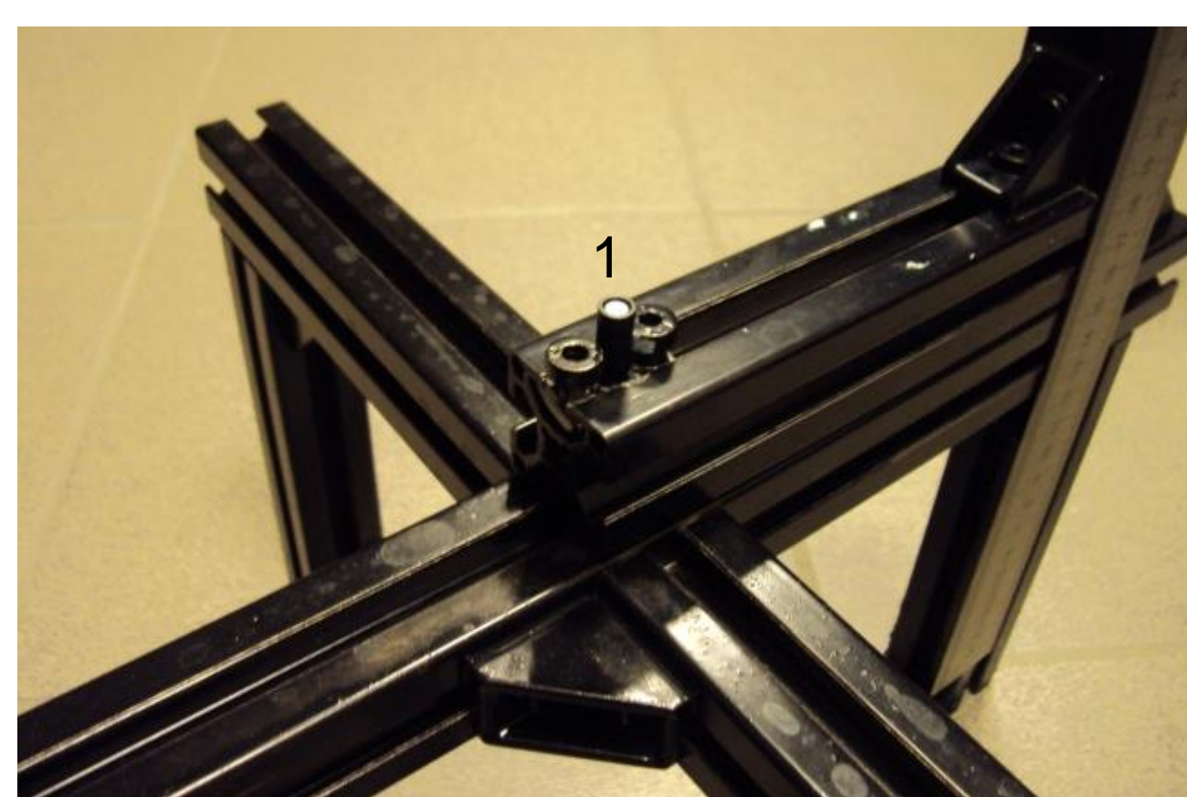
The set-up showing the irradiance probe (1), the optical fibre (2) and spectrometer (3) attached to the frame. The four legged support structure is not part of the set-up, during experiments the frame is detached from the support structure.
