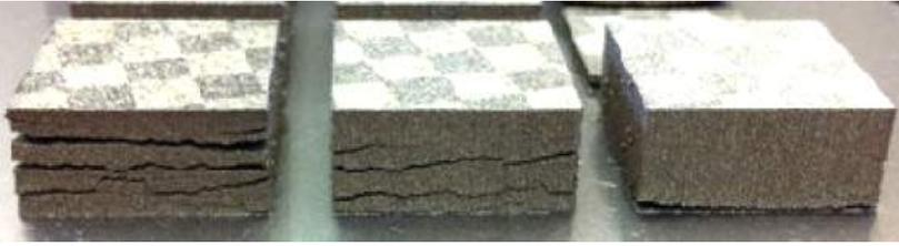
Figure 3.14: Cracks in SLM produced M2 High Speed Steel, using a preheating of 100°C and 90W laser power. From left to right, the scan speed equals 250mm/s, 400mm/s and 550mm/s [221].
