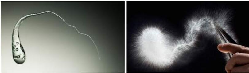
Figure 1.8: Prince Rupert's drop: a tadpole shaped, quenched glass droplet that resists hammer blows to the thicker part, but is extremely sensitive to disturbances of the tail. Release of the strain energy (residual stresses) causes the drop to explode.
