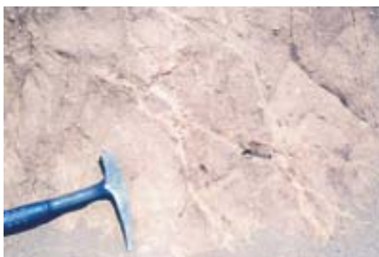
Figure 9: Conjugate fracture set, filled with sandy material in the Quaternary alluvial deposits (hammer = 33 cm long) (site situated some 100 m SE of site 18; Figure 4).
