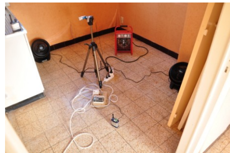
FIG 4. Co-heating test equipment: heat sources controlled by thermostats, ventilators, temperature sensors and pulse meters spread throughout the investigated dwelling. Sensor data (including weather station data) is transmitted to a central logger located on site.
