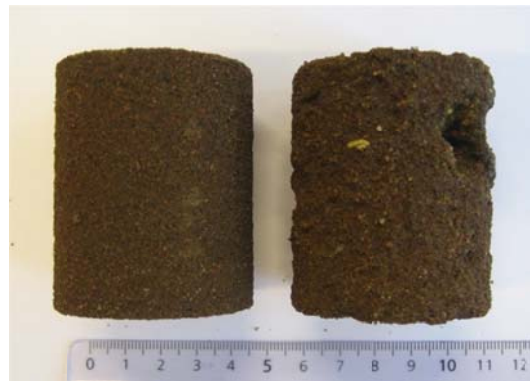
Fig. 3. Test sample of “high” (left) and “low” (right) quality Diestian ferruginous sandstone.
