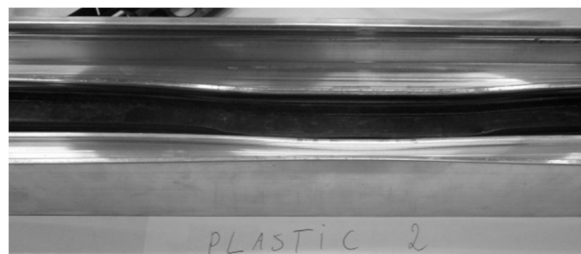
Fig. 16: Failure mode of the support blocks
