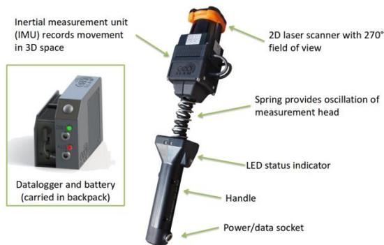
Figure 3: ZEB1 device image from <http://www.3dlasermapping.com/>
