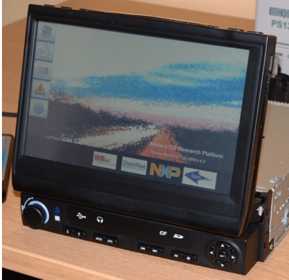
Figure 5.7: Example of an on-board-unit installed in trucks.
