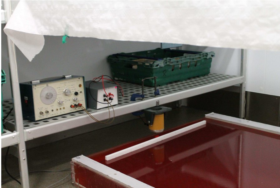
Figure 2: The experimental setup, consisting of a plexiglass tank filled with gelatine, an expanded polystyrene beam, and a harmonic shaker.
