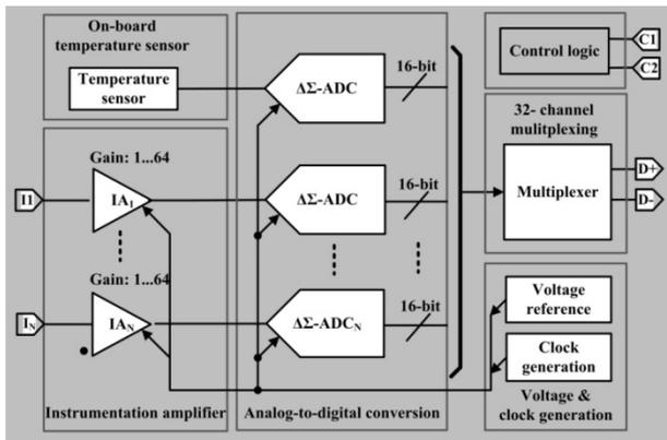
Figure 2: System diagram of the Sensor Instrumentation SoC
