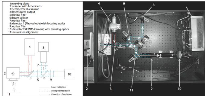
Figure 2 Optical set-up of SLM machine.
