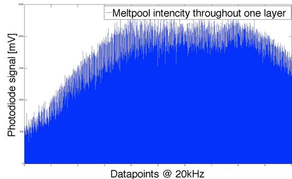
Figure 4 Melt pool intensity throughout one layer
