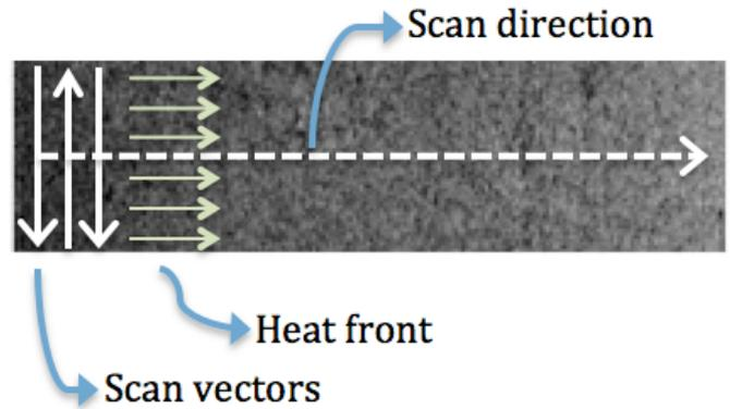
Figure 3 Melt pool intensity map of one layer
