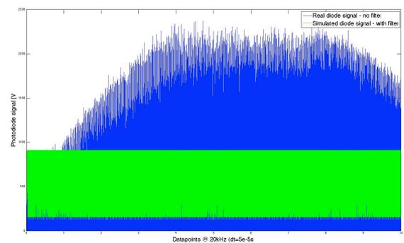
**Figure 7 Melt pool intensity throughout one layer**
