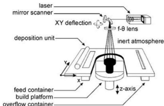
Figure 1 Schematic overview of the SLM process
