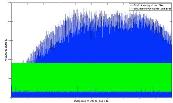
Figure 7 represents the melt pool intensity throughout one layer with and without control. It can be seen that, with control, the average intensity does not change anymore throughout one layer in comparison to the uncontrolled setup.
