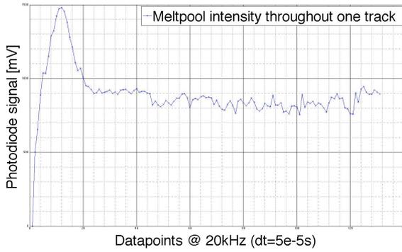
**Figure 5 Melt pool intensity throughout one scan track**
