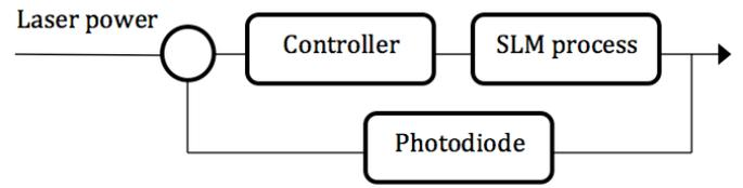
**Figure 6 Schematic overview of feedback controller**
