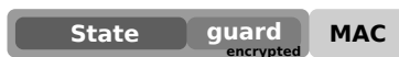
Figure 4.3: Stored states are confidentiality and integrity protected. Freshness is based on the enclosed guard.
