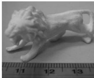
(b) 3D sintered  $\text{Al}_2\text{O}_3$  part
