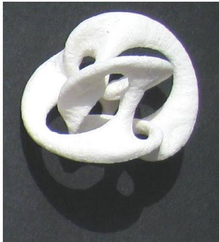
Figure 4: Example of a freeform shaped alumina part obtained through indirect SLS®.
