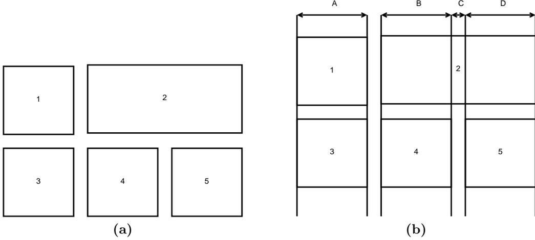
**Figure 6:** Converting linear load constraints over positions 1-5 (a) to cumulative load constraints by considering uniform sub-areas A,B,C and D (b).
