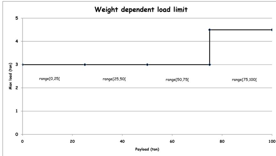
**Figure 5:** Position slot with multiple load limits, depending on the payload of the aircraft (*multiweight* position slot).
