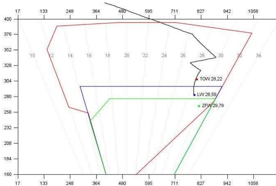
**Figure 4:** Graphical representation of the CG limits. The horizontal axis shows the longitudinal coordinate of the CG (in inches from the datum), the vertical axis shows the weight of the aircraft (in lbs.). The inner, outer and middle regions show the limits for the CG and the weight of the aircraft during loading (ZFW), take off (TOW) and landing (LW). The black line indicates the change of the aircraft's weight and CG during the different stages of flight.
