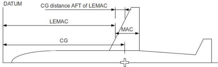
**Figure 7:** Graphical representation of the Mean Aerodynamic Chord (MAC) and the Leading Edge MAC (LEMAC).
