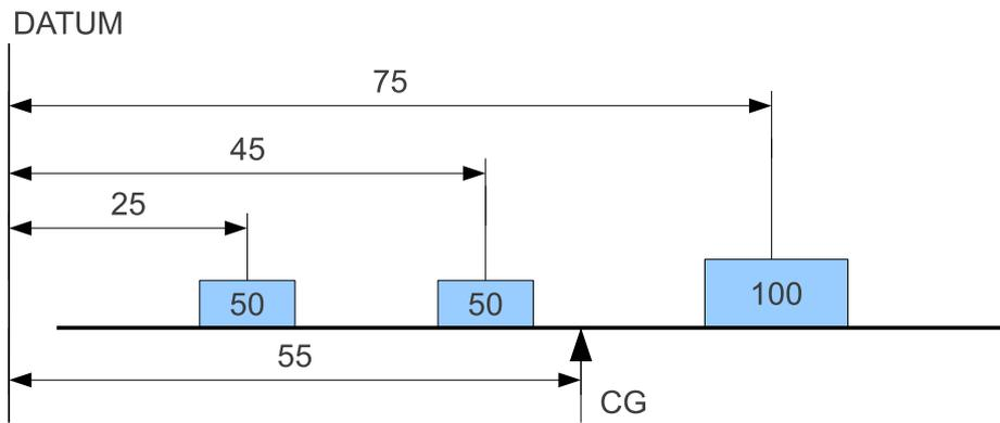
**Figure 3:** Graphical representation of a CG calculation. The three loads of 50, 50 and 100 exert a gravitational force on the surface, which can be virtually replaced by a fictitious load of 200 positioned at the CG  $\left(= 55 = \frac{25 \cdot 50 + 45 \cdot 50 + 75 \cdot 100}{50 + 50 + 100}\right)$ . Alternatively, the CG also represents the position on the surface where the three loads would be perfectly balanced.
