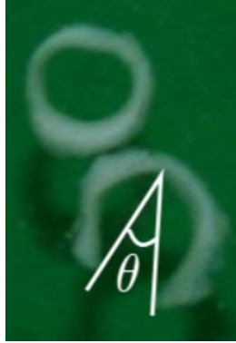
Figure 5: opening angle \theta , quantifying the residual strain in circumferential direction (79)
