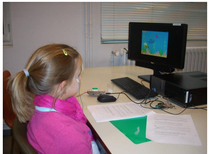
Fig. 5: EOG-based human-computer interface controlling a computer game was developed during a workshop for 10-12 year olds.
