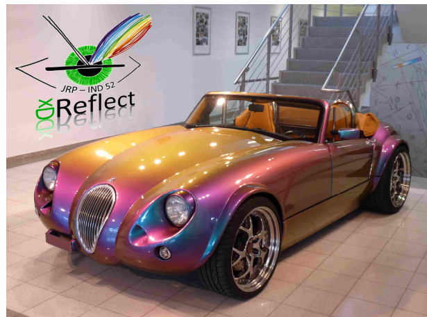
Figure 1. Car painted with a goniochromatic varnishing, according to the visual perspective and the light conditions, the colour impression changes.
