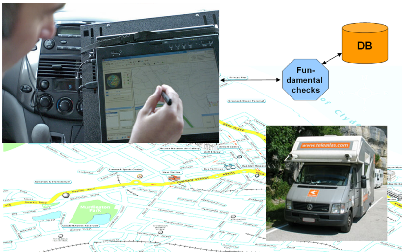
Figure 2.1: Geographic data collection with mobile mapping vehicles
