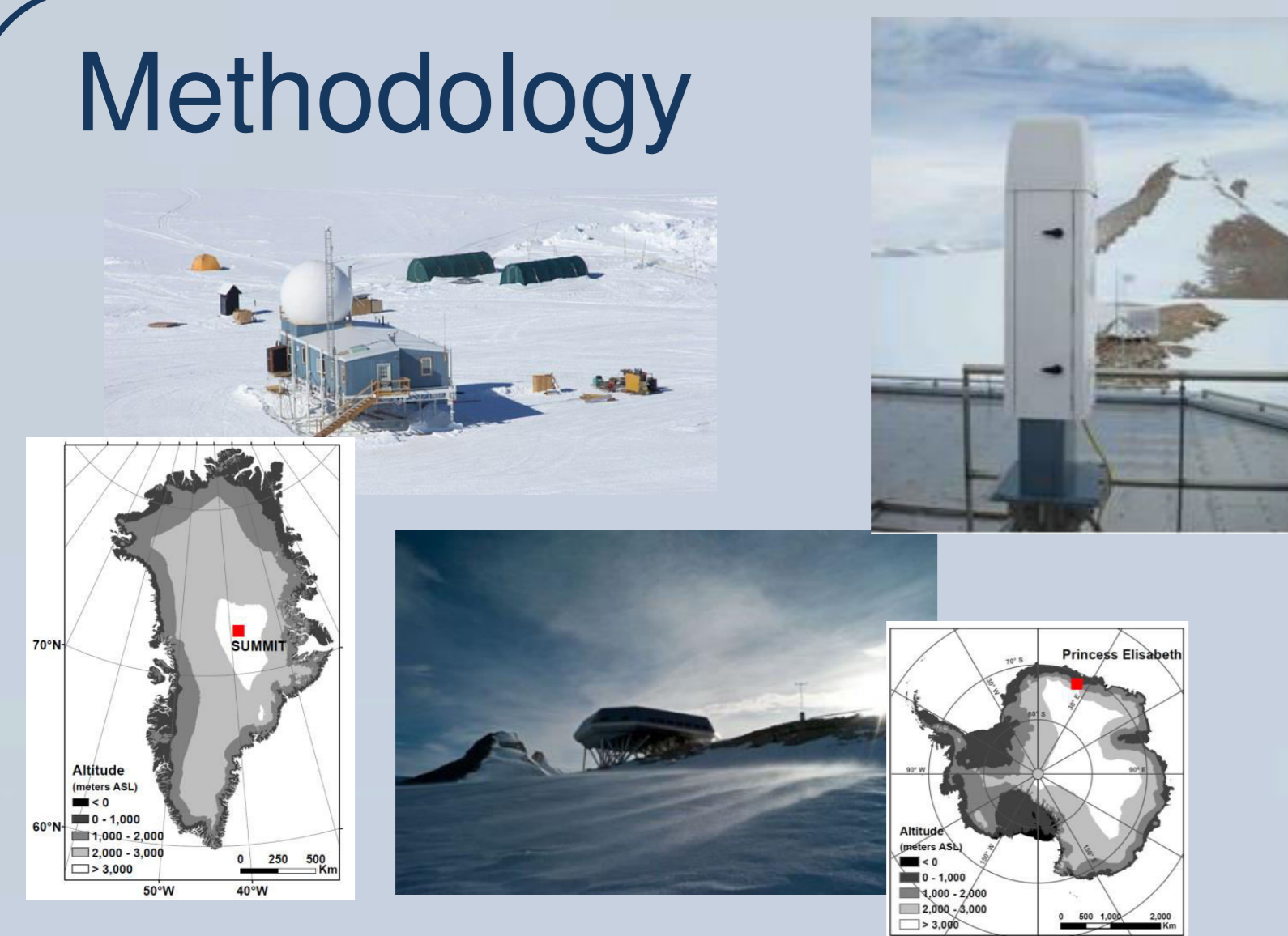
Fig. 1: Ceilometers Vaisala CL31 at Princess Elisabeth, Antarctica and CT25K at Summit, Greenland provide ground-based cloud observations
