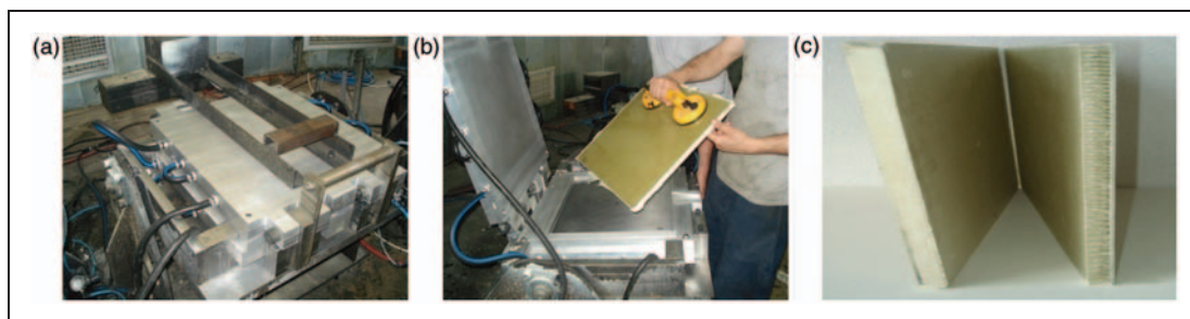
Figure 3. Fabrication steps of foam filling process (a and b) and view of foamed and unfoamed panels (c).
