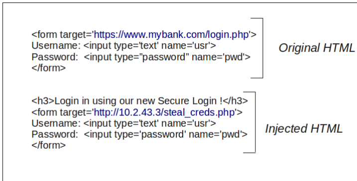
Figure 7.2: Example of an injected HTML form by a MITM attacker
