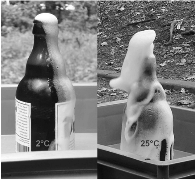
Fig. 1. The visual effect of beverage temperature on the gushing volume. Left, at 2°C only 10 g are expelled from a 330 mL bottle and right, at 25°C, 132 g are expelled from a 330 mL bottle of the same brand.
