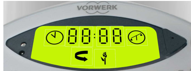
Figure 8 The display of the product is made up of nine rectangular patches with different textures that are changed at run time by the simulator.
