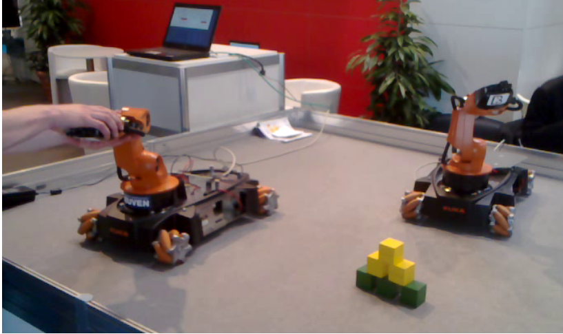
Figure 7.1: Bidirectional youBot coupling demonstration: each robot copies the cartesian position of its peer robot.
