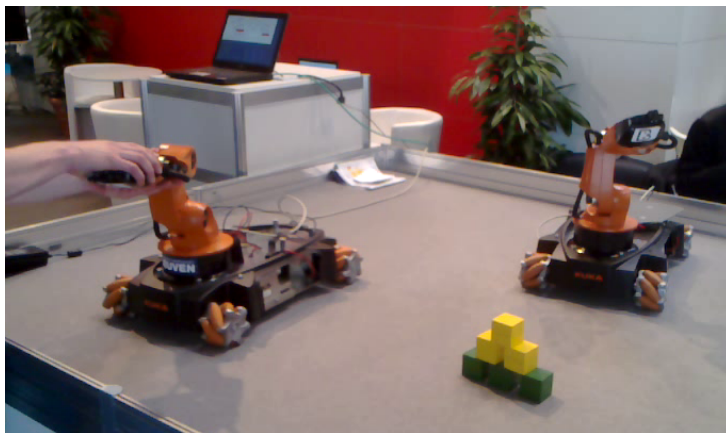
Figure 4.17: The youbot coupling demo at the Automatica trade fair. The forces of pulling on one robot arm are felt on the other side. Once the forces rise above a threshold, the coupling is disabled and both robot arms are put into floating mode.
