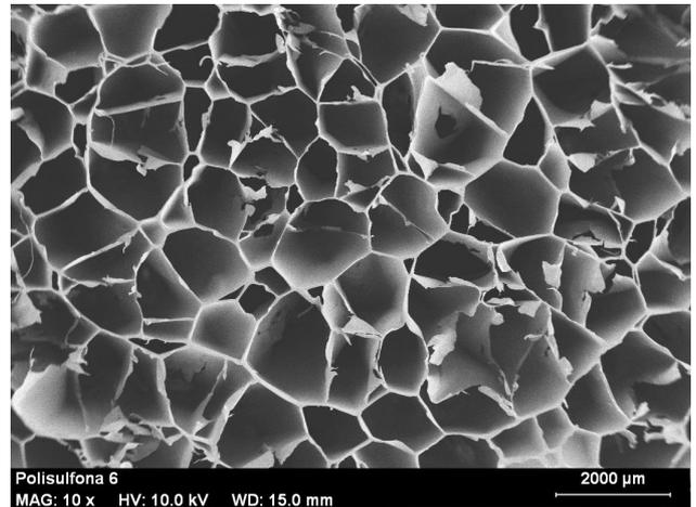
**Fig.6.** SEM micrograph of the anisotropic PES foam looking straight down through the length of the cells. Note the difference in scale between the PES and EPS micrographs.
