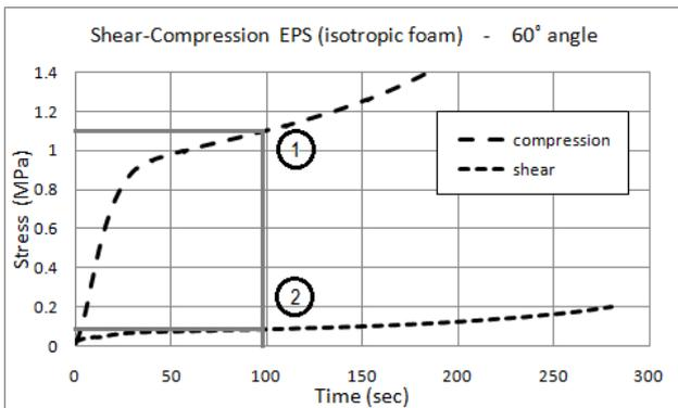
**Fig.8.** 60° shear-compression test of helmet grade EPS. The analysis is carried out until one of the curves reaches a critical value; in this case, the compressive curve reaches the biomechanical limit of 1.12 MPa at point (1). The corresponding point in time in the shear curve is determined, point (2).
