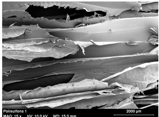
**Fig.7.** SEM micrograph of anisotropic PES foam looking along the length of the cells.
