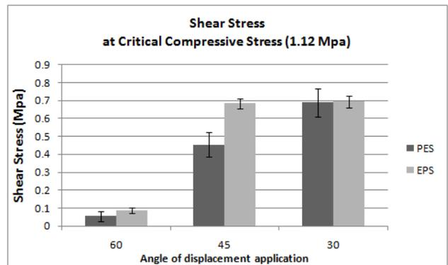
**Fig.17.** Shear stress when the compressive stress reaches the critical value of 1.12 MPa.
