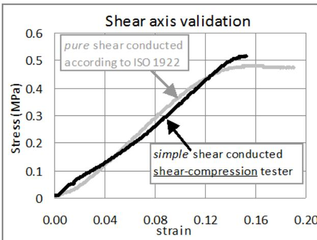
**Fig.4.** Shear test results for the validation of the new test setup. The close correlation of the data obtained from the shear axis of the shear-compression tester (black) and the data obtained in a calibrated Instron tester according to ISO 1922 (grey), is within experimental sample scatter, and thus the acquired data is considered to be accurate in the shear axis.
