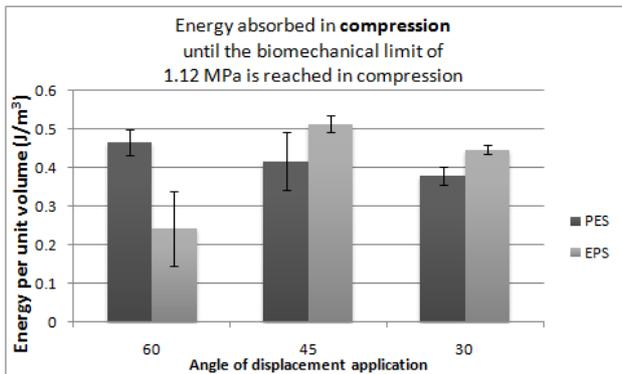
**Fig.14.** Energy absorbed in the foam material by compression for both materials, over 3 different angles of displacement.
