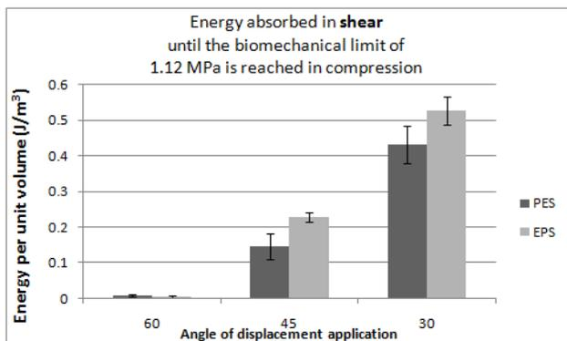
**Fig.15.** Energy absorbed in the foam material by shear for both materials, over 3 different angles of displacement.
