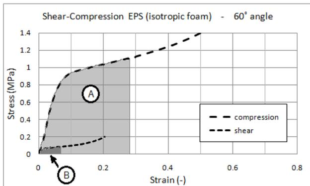
**Fig.9.** Points (1) and (2) are located on the stress-strain curve, and material properties can be determined at or until these points. For this analysis, the area under the curve, or the absorbed energy, was of interest. Areas (A) and (B), corresponding to the energy absorbed until points (1) and (2) were determined.
