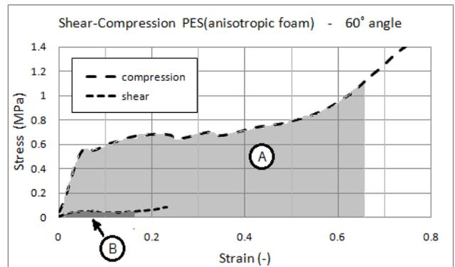
**Fig.11.** The areas under the curves, (A) and (B) are determined, indicating the energy that is absorbed in compression and shear up until points (1) and (2).
