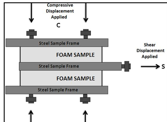
Fig.1. Graphical representation of the sample frame for shear-compression testing.
