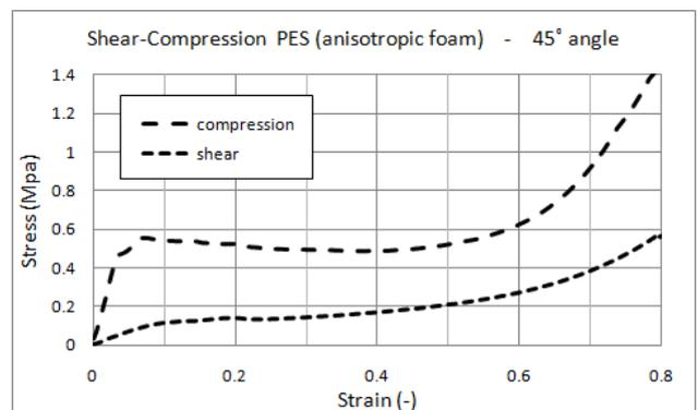
**Fig.13.** Compressive and Shear stress vs. strain curves for the PES material at an applied displacement angle of 45°. The plateau stress of PES at 45° is slightly lower than that it was at 60°. The shear resistance is higher at 45° than at 60°, however, at 45° the shear resistance of PES is still lower than the EPS material at 45°.
