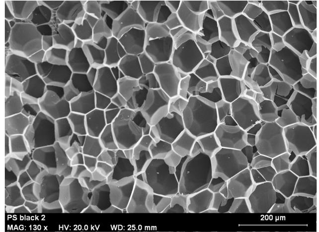
**Fig.5.** PES micrograph of isotropic EPS foam. The backs of the cells are visible here, unlike in figure 3.
