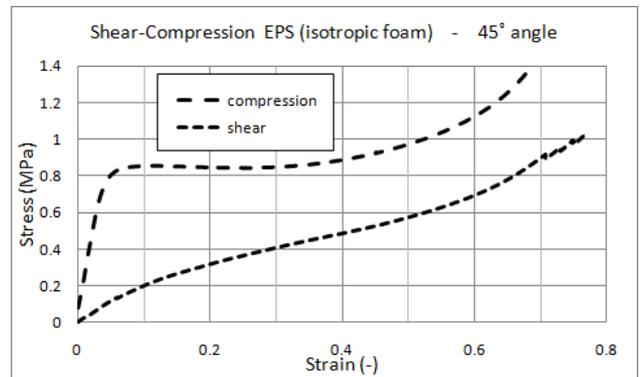
**Fig.12.** Compressive and Shear stress vs. strain curves for the EPS material at an applied displacement angle of 45° (equal rates of shear and compression displacement). The plateau stress of EPS at 45° is lower than that at 60°; however the shear resistance is much higher at 45° than at 60°.
