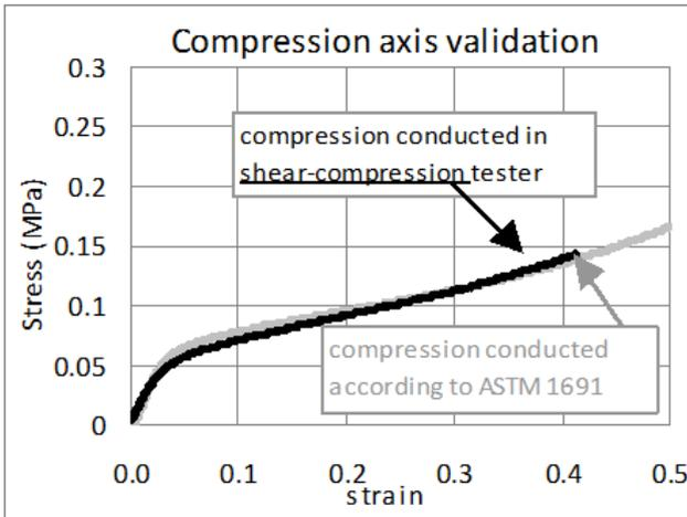
**Fig.3.** Compression test results for the validation of the new test setup. The close correlation of the data obtained in the compressive axis of the shear-compression tester (black) and the data obtained in a calibrated Instron tester according to ASTM 1691 (grey), is within experimental sample scatter, and thus the acquired data is considered to be accurate in the compressive axis.
