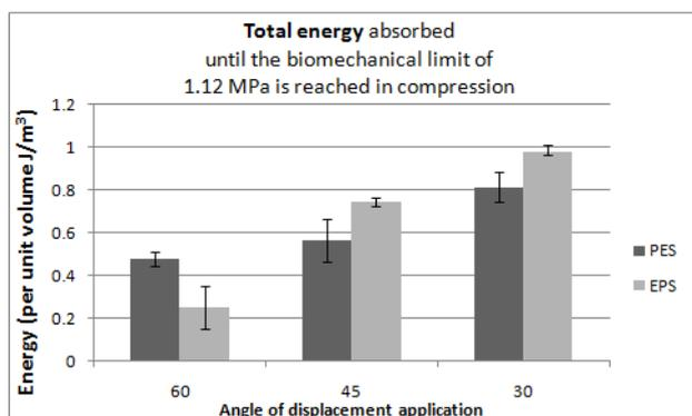
**Fig.16.** Total energy (from compression and shear) absorbed in the foam material for both materials, over 3 different angles of displacement.
