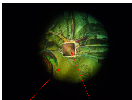
Unsatisfactory greenish black coloured Cr-black coating
