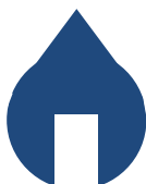
Top View: CS of solid microneedle with slit along its entire height
