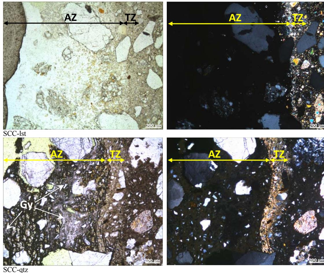
Figure 4: Polarizing light microscopic images of SCC-1st and SCC-qtz with parallel polarising (left) and crossed polarising (right) show the extent of damage induced by chemical attack of sulphuric acid (AZ: attacked zone; TZ: transition zone; Gy: gypsum)
