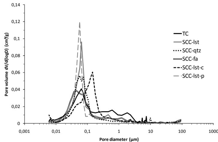
Figure 1: Pore volume of the unexposed concrete specimens.
