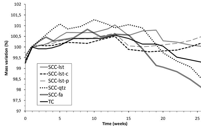
Figure 2: Mass variation in SCC mixtures and TC during continuous immersion in sulphuric acid solution.
