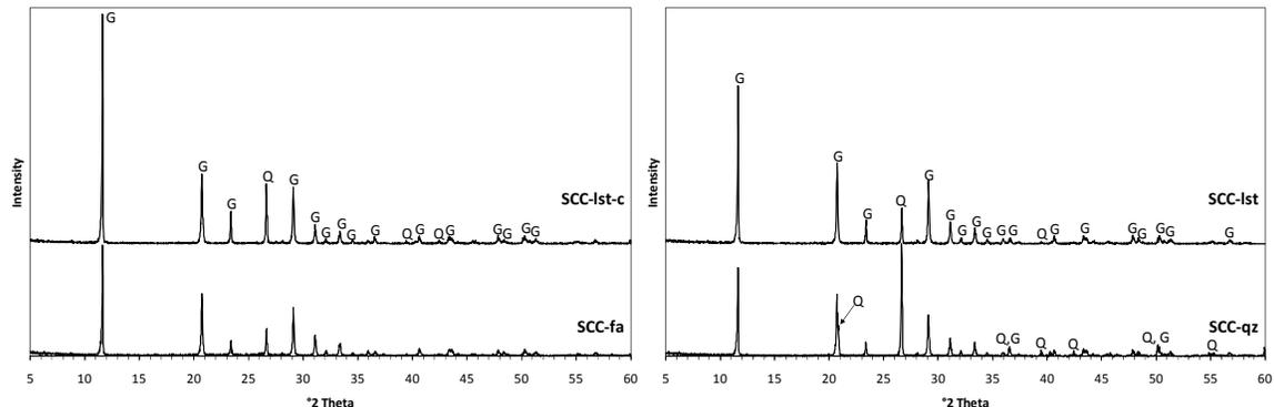
Figure 3: XRD patterns of the attacked zone of the SCC specimens (G: gypsum; Q: quartz).
