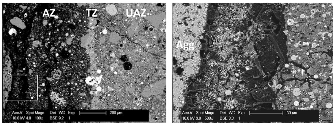
Figure 5: SEM micrographs showing a dense transition zone (TZ) between attacked zone (AZ) and unattacked zone (UAZ) (left image), and gypsum crystals surrounding an aggregate (Agg) at the ITZ (right image as highlighted within a square in the left image) in SCC-fa.
