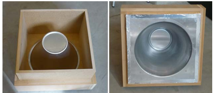
Figure 7: Mold in a box of MDF.
