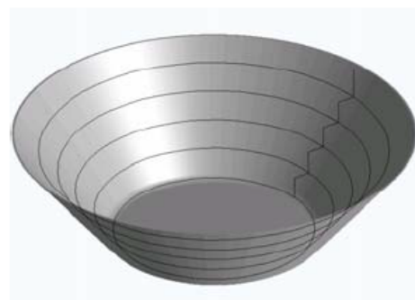
Figure 1: Single Ppoint Incremental Forming process, with example of cone. [3]
