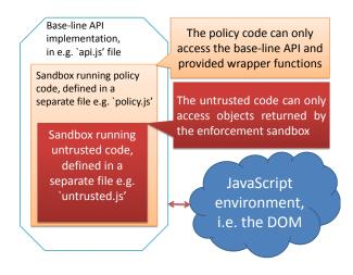
Figure 1: The two-tier sandbox architecture
