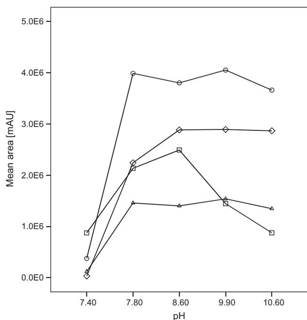
Fig. 2. Influence of the pH value of the reaction mixture on the dabsyl derivatisation yield at 70 °C with SPD (○), TYR (◇), HIS (□) and SPM (△).
