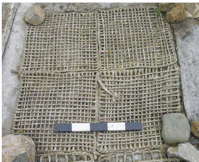
Plate V. Well preserved close-weave Buriti geotextiles after 10 months field emplacement, Rushen Abbey, Isle of Man (June 2008). This figure is available in colour online at wileyonlinelibrary.com/journal/ldr .
