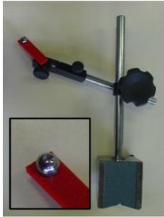
Figure 8 Sphere holder with socket
