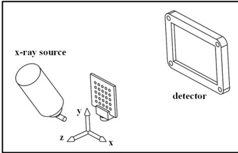
**Figure 3 Setup of the holes plate inside the XCT machine**
