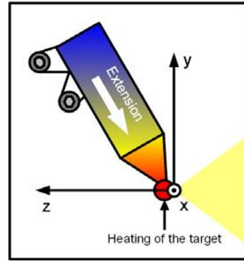
**Figure 7 X-ray source mounting**
