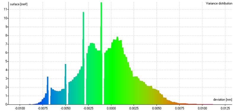
**Figure 13 Histogram of the deviation between the two reconstructions; with and without drift compensation**
