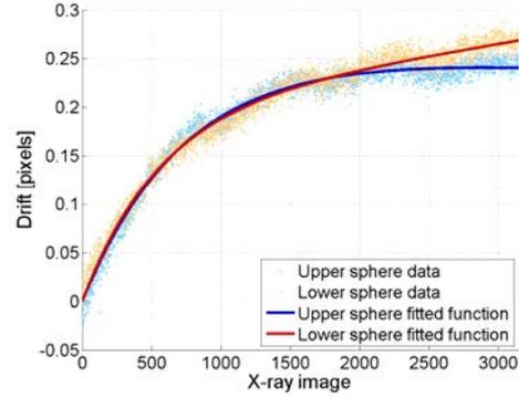
**Figure 11 Shift of the spheres in y- direction**
