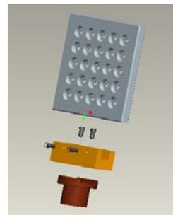
Figure 2 Exploded view of the hole plate clamping
