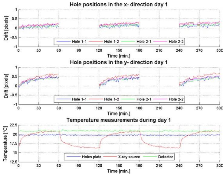
**Figure 5 Drift of the 4 holes on the 2D X-ray images and temperature measurements**
