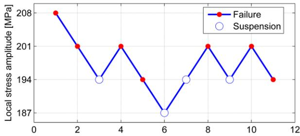
Figure 4. Staircase method for k<sub>t</sub> = 2
