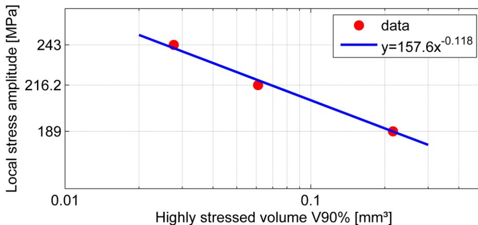
Figure 7. Local stress amplitude vs highly stressed volume
