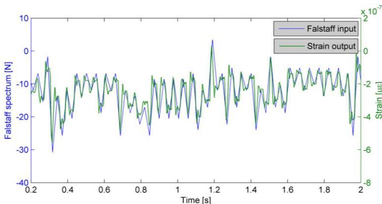
Figure 9. Falstaff load spectrum and measured strains
