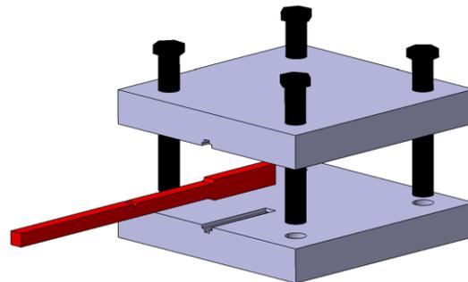
Figure 3. Specimen clamping tools
