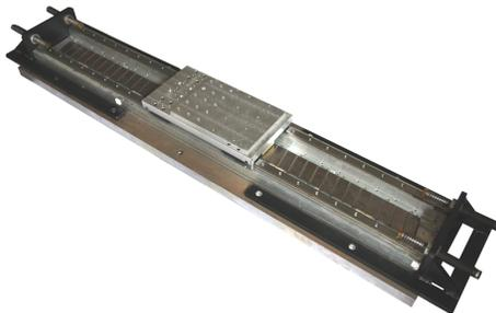
Figure 3.4: Picture of the linear motor drive test-setup in the PMA-lab at KULeuven.
