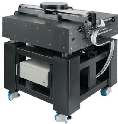
Figure 4.1: Experimental test setup of a linear motor with airbearings.
